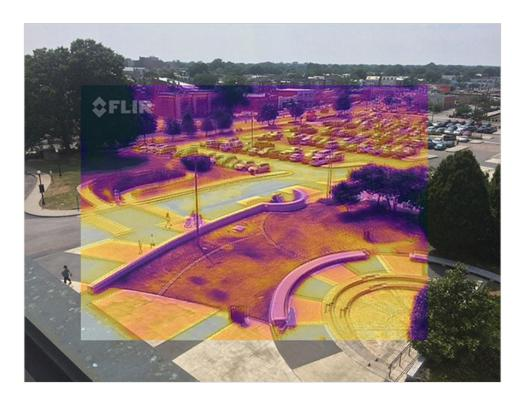
The inset image, taken with a forward looking infrared (FLIR) camera, shows heat and is overlain on a regular photograph for context. In the FLIR image, lighter or brighter colors indicate warmer areas, while darker areas are cooler.
